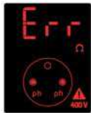
Connection between phases under 400 V.
