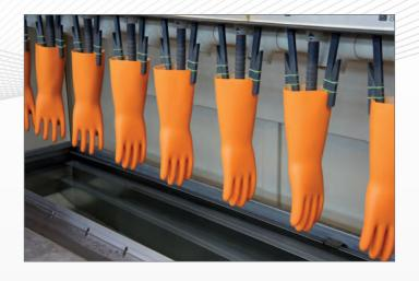
Classed in category III of Personal Protective Equipment, the electric insulating gloves are treated in compliance with international standards that require strictly defined conformity.
